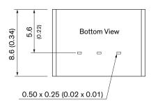
Dimensions in mm (inch) Tolerances:  $x.xx \pm 0.5 (\pm 0.02)$ Tolerances:  $x.xxx \pm 0.25 (\pm 0.01)$
