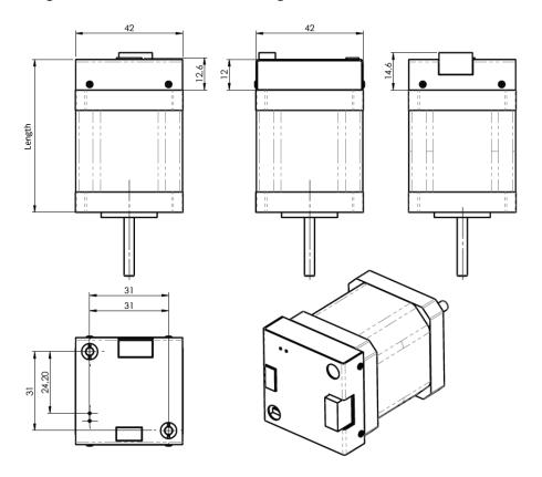
Figure 1: PD42-x-1670 overall dimensions in mm
