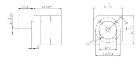
Figure 2: Motor without electronics - all dimensions in mm
