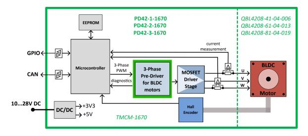
Figure 6: PD-x-1670 block diagram
