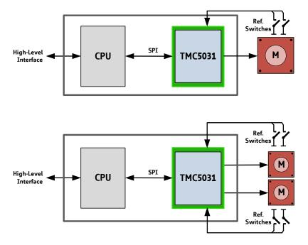
Two reference switch inputs can be used for each motor. A single CPU controls the whole system, which is highly economical and space saving.
