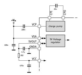
Figure 3.6 Adding an RC-Filter on VCC for reduced ripple
