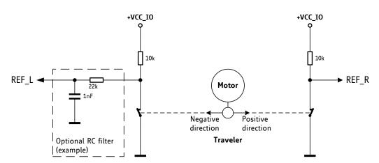
Figure 9.4 Using reference switches (example)
