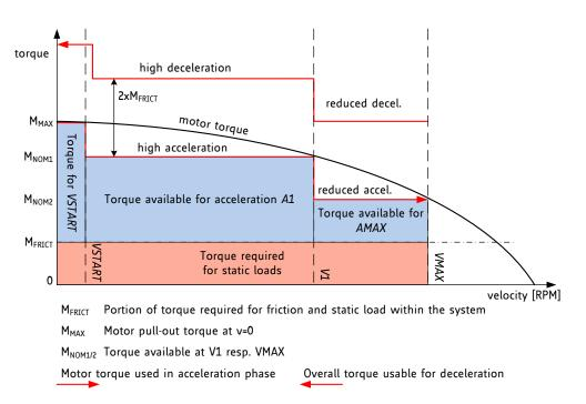
Figure 9.2 Illustration of optimized motor torque usage with TMC5031 ramp generator
