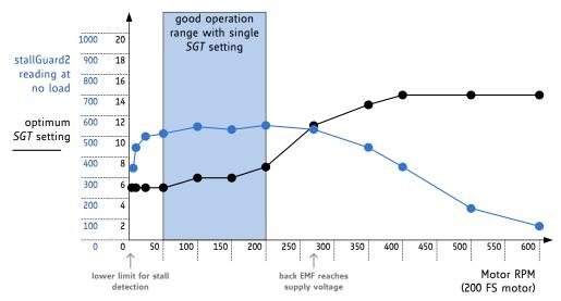
Figure 10.2 Example: Optimum SGT setting and stallGuard2 reading with an example motor
