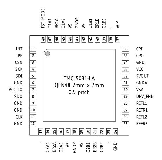
Figure 2.1 TMC5031 pin assignments.
