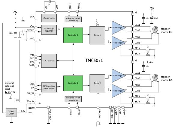
\* For a reliable start-up it is essential that VCC\_IO comes up to a minimum of 1.5V before the TMC5031 leaves the reset condition. Therefore, TRINAMIC recommends using a fast-start-up voltage regulator (e.g. TS3480CX33) in a 3.3V environment.
