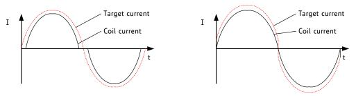
Coil current does not have optimum shape
