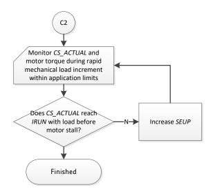
Figure 13.3 Enabling coolStep (in combination with spreadCycle)
