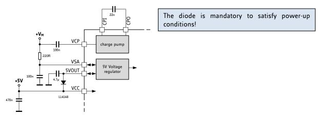
Figure 3.4 Using an external 5V supply to reduce linear regulator power dissipation
