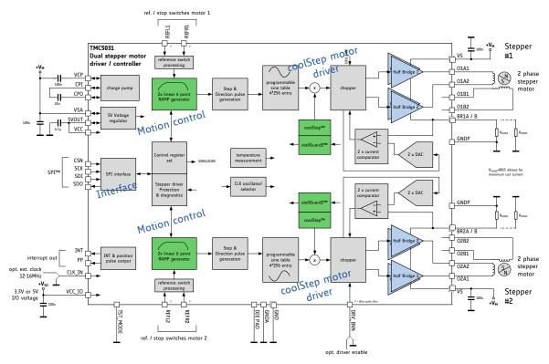
Figure 1.1 Basic application and block diagram
