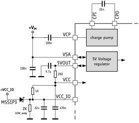
Figure 3.2 External supply of VCC\_IO (showing optional filtering for VCC)
