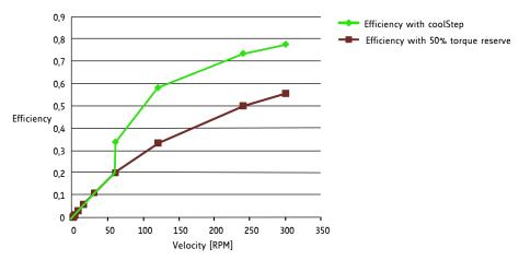
Figure 1.2 Energy efficiency with coolStep (example)
