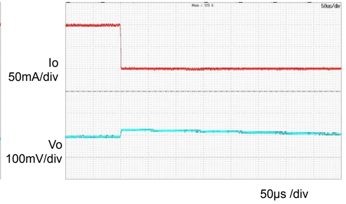
Figure 11. Transient Response ( T_a=-40^\circ\text{C} ) ( I_o = 0.1\text{A} \rightarrow 0\text{A} )
