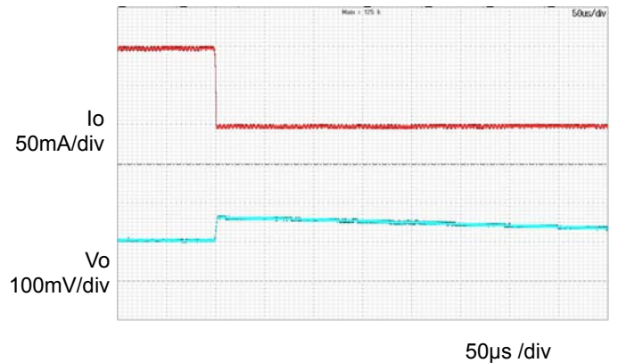
Figure 13. Transient Response ( T_a=105^\circ\text{C} ) ( I_o = 0.1\text{A} \rightarrow 0\text{A} )
