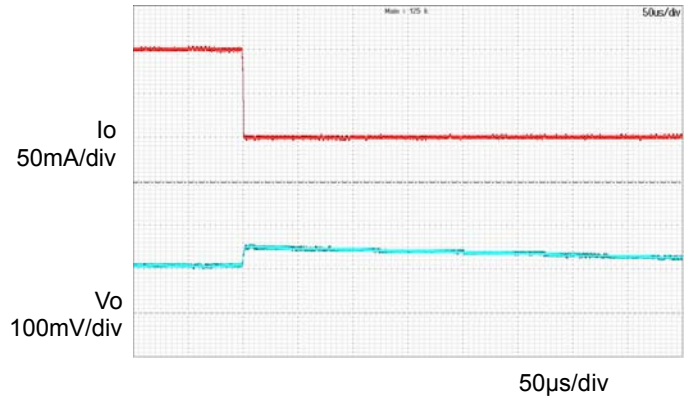
Figure 9. Transient Response ( T_a=25^\circ\text{C} ) ( I_o = 0.1\text{A}\rightarrow 0\text{A} )
