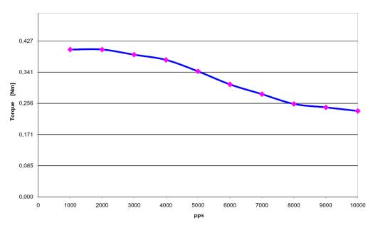
Figure 5.4: QSH4218-47-28-040 speed vs. torque characteristics
