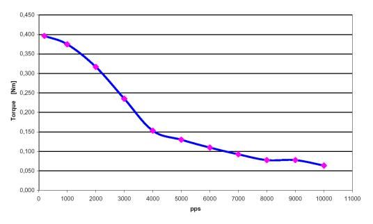
Figure 5.3: QSH4218-51-10-049 speed vs. torque characteristics
