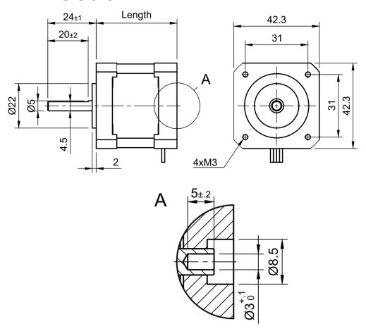
Figure 4.2: Dimensions (all values in mm)
