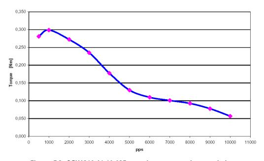
Figure 5.2: QSH4218-41-10-035 speed vs. torque characteristics
