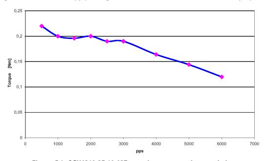
Figure 5.1: QSH4218-35-10-027 speed vs. torque characteristics
