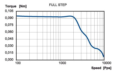
Figure 5.2: QSH2818-51-07-012 speed vs. torque characteristics
