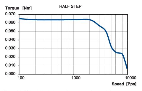
Figure 5.1: QSH2818-32-07-006 speed vs. torque characteristics
