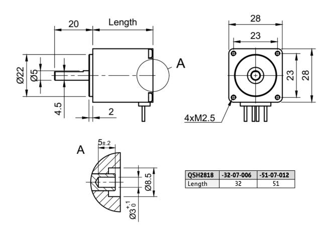
Figure 4.2: Dimensions (all values in mm)
