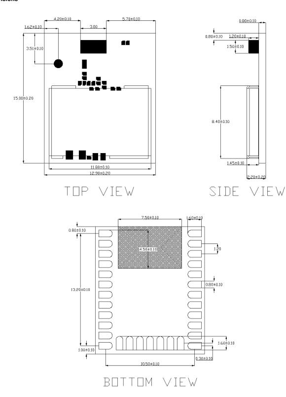
Figure 8.1. Module Dimensions
