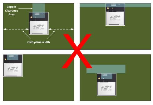
Figure 7.2. Non-Optimal Layout Examples
