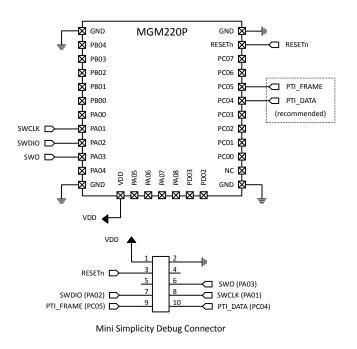
Figure 5.2. Stand-Alone SoC Configuration
