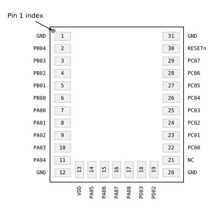
Figure 6.1. 31-Pin PCB Module With LF Crystal Device Pinout
