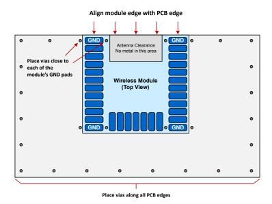
Figure 7.1. Recommended Layout for MGM220P
