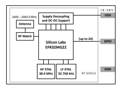
Figure 3.1. MGM220P Block Diagram
