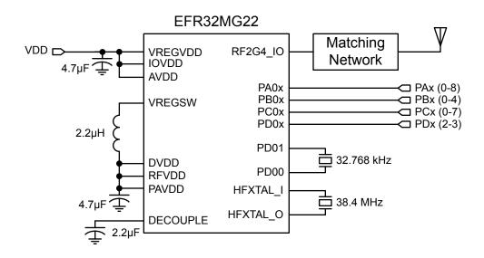
Figure 3.2. MGM220P Module Schematic
