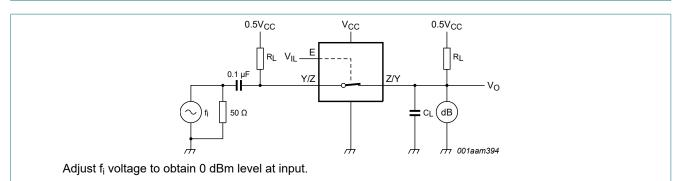
Fig. 19. Test circuit for measuring isolation (OFF-state)
