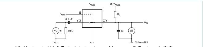
Adjust f<sub>i</sub> voltage to obtain 0 dBm level at output. Increase f<sub>i</sub> frequency until dB meter reads -3 dB.
