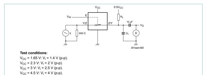
Fig. 17. Test circuit for measuring total harmonic distortion
