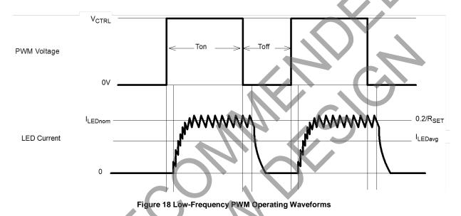
There are different ways of accomplishing PWM dimming of the AP8801 LED current:
