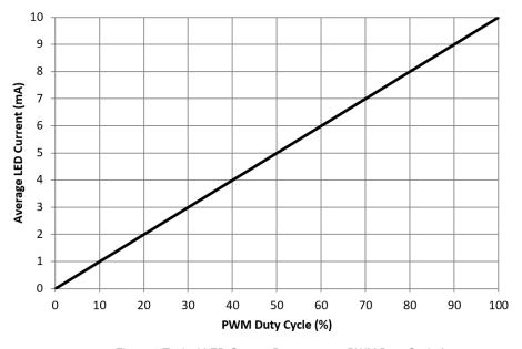
Figure 4 Typical LED Current Response vs. PWM Duty Cycle for 25kHz PWM Frequency (Dimming Range 200:1)
