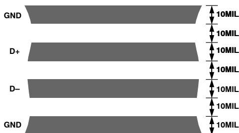
Figure 34. Arrangement of Signal Tracks
