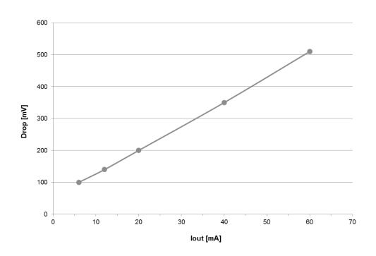
Figure 5. Channel dropout voltage vs output current (Tj = 25 °C)
