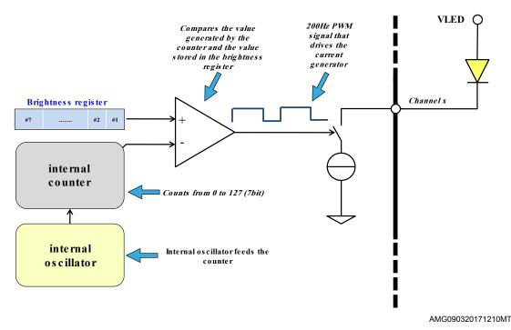
The ALED1262ZT implements 128 non-linear dimming steps to adequate LED brightness change to human eye light perception, giving in this way the impression of brightness linear variation. The exponential law used to calculate the dimming steps is the following:
