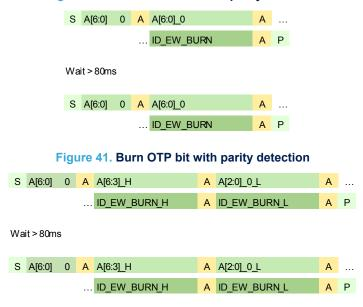
Figure 40. Burn OTP bit without parity detection
