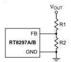
Figure 1. Output Voltage Setting
