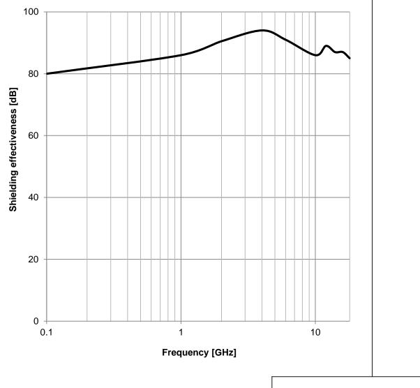
CHECKED REVISION DATE (YYYY-MM-DD) GENERAL TOLERANCE PROJECTION METHOD ViMa 005.003 2020-03-06 DIN ISO 2768-1m DESCRIPTION **WE-LT Conductive Shielding** Würth Elektronik eiSos GmbH & Co. KG Gasket ORDER CODE EMC & Inductive Solutions Max-Eyth-Str. 1 3020402 74638 Waldenburg Germany SIZE/TYPE STATUS Tel. +49 (0) 79 42 945 - 0 www.we-online.com BUSINESS UNIT PAGE WÜRTH ELEKTRONIK 2/3 eiSos Valid Square eiSos@we-online.com
