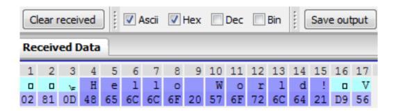
Thus the CMD\_DATAEX\_IND message informs us that we received a packet with payload of 0x0D (13) bytes. 12 byte of these are user payload (0x48 0x65 0x6C 0x6C 0x6F 0x20 0x57 0x6F 0x72 0x6C 0x64 0x21 = Hello World!) and one byte is the RSSI value (here 0xD9, which is two's complement for -39 dBm) directly outputted behind the payload, before the checksum.
