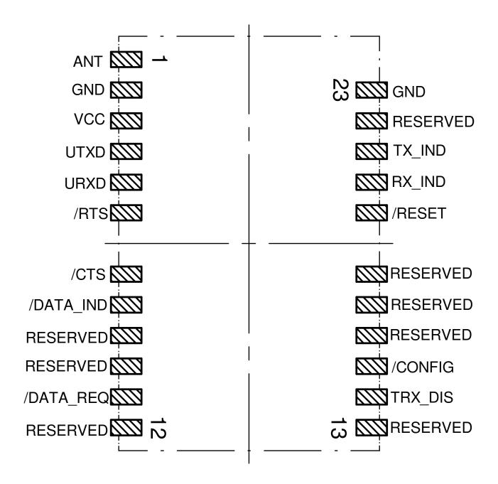
Figure 2: Pinout
