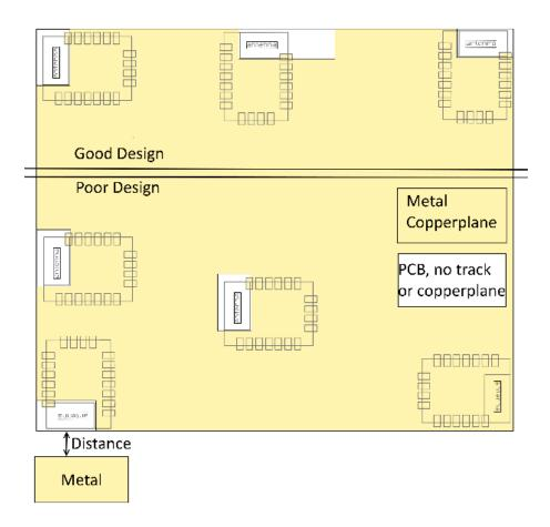
Figure 11: Placement of the module with integrated antenna
