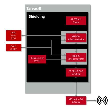
Figure 1: Block diagram
