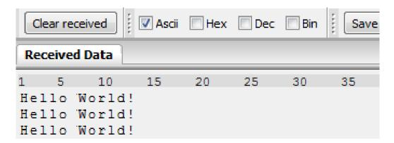
You just used the so called "transparent mode" of the modules to send your data. The address mode that was used is "0". Thus all radio frames are broadcasts that can be received by anyone listening with an Tarvos-II in default settings. The frame you send was generated using the timeout method.
