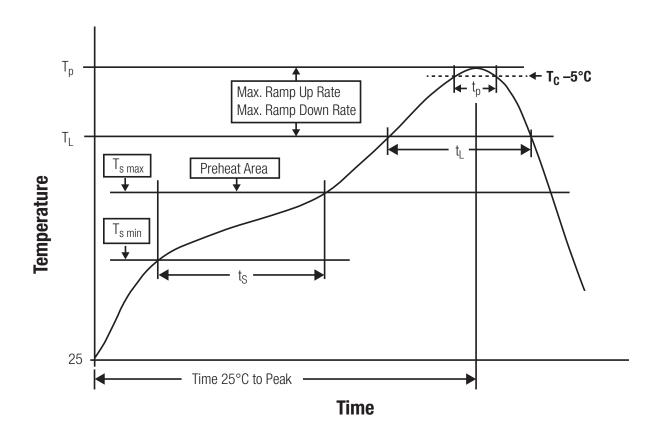
Figure 20: Reflow soldering profile
