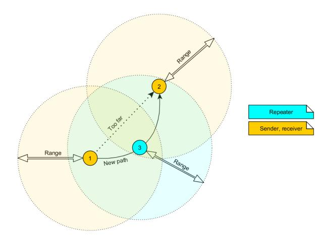
Figure 8: Range extension using repeaters
