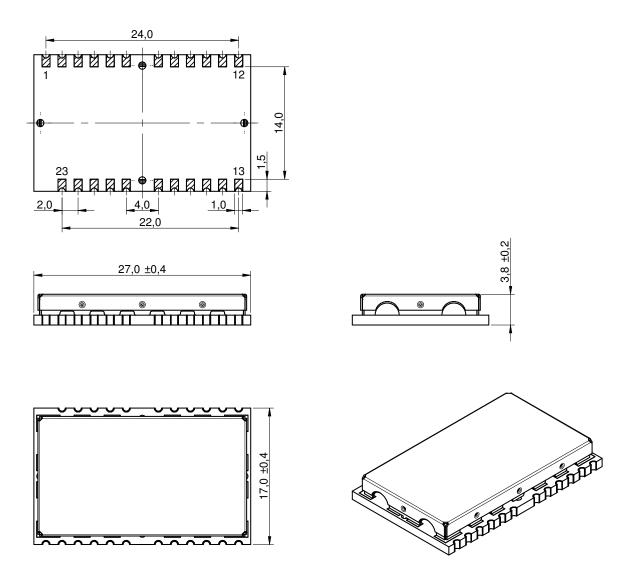
Figure 21: Module dimensions [mm]
