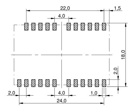
Figure 22: Footprint and dimensions [mm]
