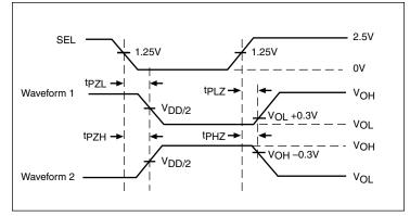
**Voltage Waveforms Propagation Delay Times**
