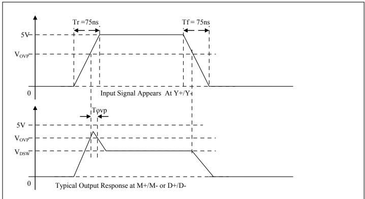
The PI3USB102G offers over voltage protection for the Y+/Y- pins to protect from shorts to VBUS (5V). When the voltage on Y+/Y- exceeds  $V_{OVP}$ , the voltage at M+/M- and D+/D- is clamped to  $V_{DSW}$  within the time  $T_{OVP}$ . For rise time of 75 ns (as per USB1.1 and USB2.0 low-speed specifications),  $T_{OVP}$  is typically 40 ns.  $T_{OVP}$  is smaller for faster risetimes. For example,  $T_{OVP}$  is typically 20 ns for rise time of 5 ns.
