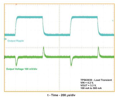
Figure 5. Load Step 100 mA to 500 mA
