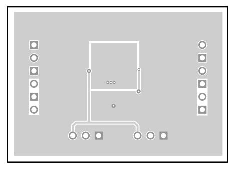
Figure 8. Bottom Layer Routing
