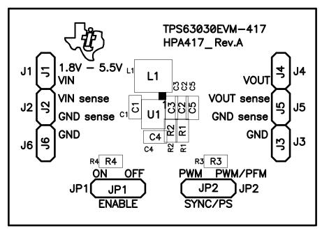
Figure 6. Assembly Layer
