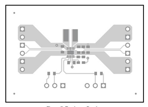
Figure 7. Top Layer Routing
