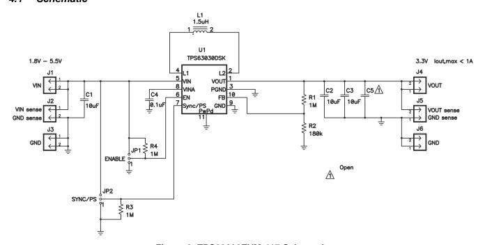
Figure 9. TPS63030EVM-417 Schematic
