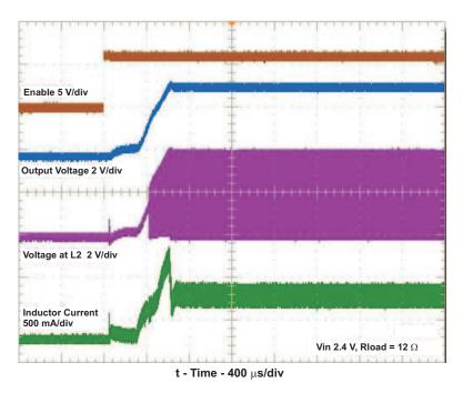
Figure 1. Turn ON into Load, Vin = 2.4 V
