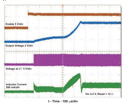
Figure 2. Turn ON into Load, Vin = 4.2 V
