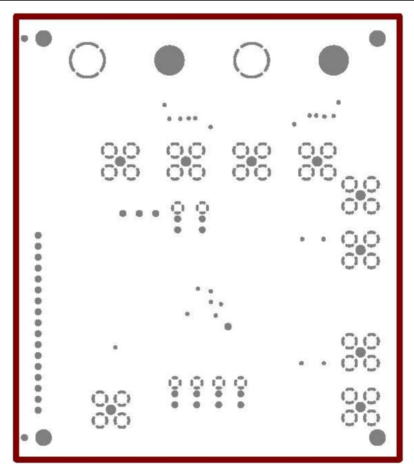
Figure 2. Layer 2, Ground Plane
