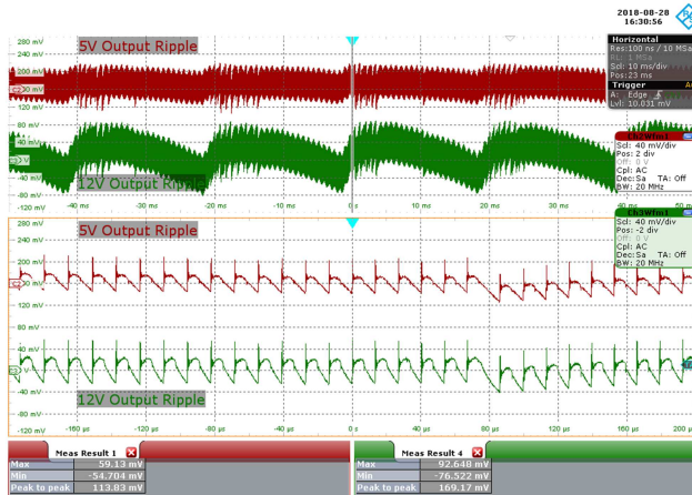
Figure 110 – 85 VAC 60 Hz, 100% Load. CH2: 5 V_{OUT} , 40 mV / div., 10 ms / div. CH3: 12 V_{OUT} , 40 mV / div., 10 ms / div. Zoom: 40 \mu s / div. 5 V Output Ripple = 113.83 mV. 12 V Output Ripple = 169.17 mV.
