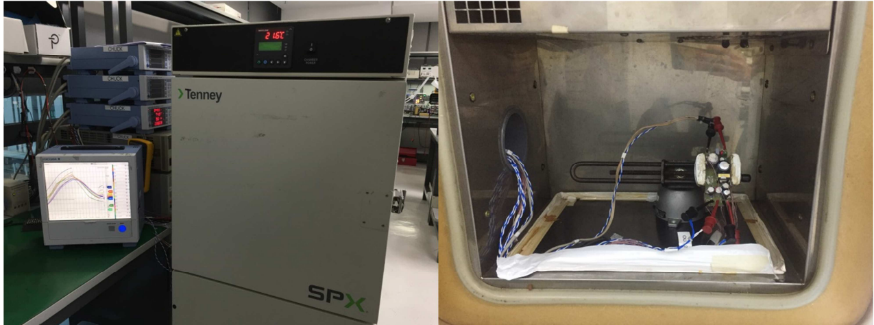
Figure 147 – Thermal Performance Set-up using Thermal Chamber.
