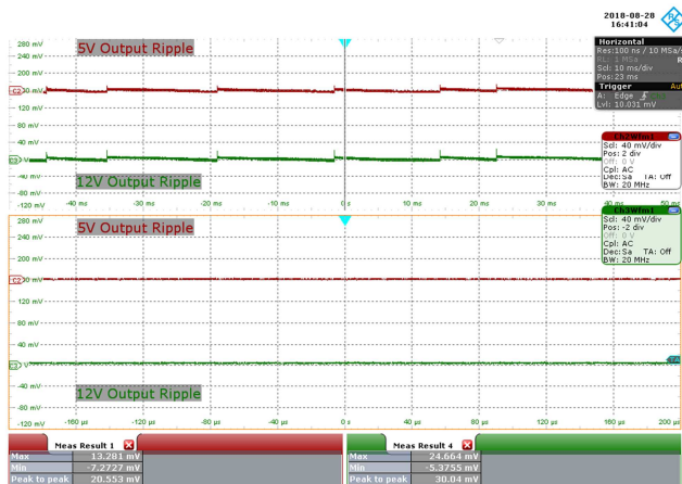
Figure 126 – 85 VAC 60 Hz, 0% Load. CH2: 5 V_{OUT} , 40 mV / div., 10 ms / div. CH3: 12 V_{OUT} , 40 mV / div., 10 ms / div. Zoom: 40 \mu s / div. 5 V Output Ripple = 17.391 mV. 12 V Output Ripple = 25.296 mV.
