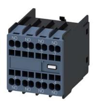
Auxiliary switch on the front, 4 NO Current path 1 NO, 1 NO, 1 NO, 1 NO for 3RH and 3RT spring-type terminal .3/.4, .3/.4, .3/.4, .3/.4
