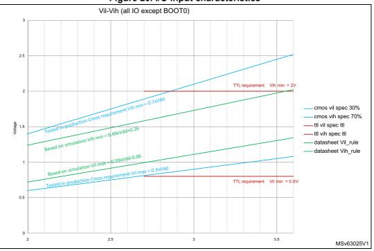
Figure 20. I/O input characteristics
