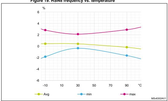
Figure 19. HSI48 frequency vs. temperature
