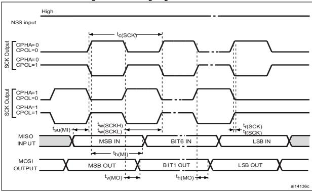
Figure 26. SPI timing diagram - master mode
