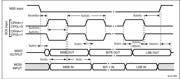
1. Measurement points are set at CMOS levels: 0.3  $V_{\text{DD}}$  and 0.7  $V_{\text{DD}}.$
