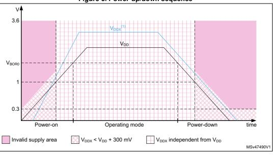
Figure 5. Power-up/down sequence
