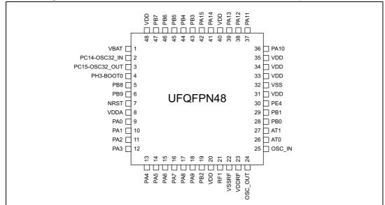
Figure 8. STM32WB50CG and STM32WB30CE UFQFPN48 pinout<sup>(1)(2)</sup>
