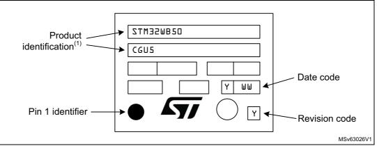
Figure 29. STM32WB50CG UFQFPN48 marking example (package top view)
