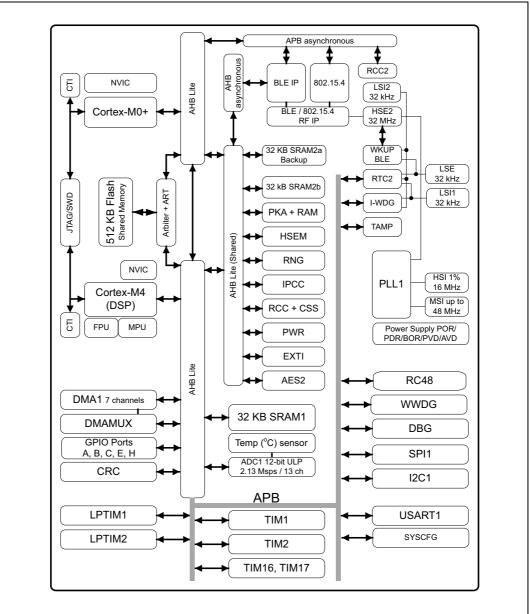
Figure 2. STM32WB30CExx block diagram
