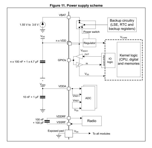
**Caution:** Each power supply pair (such as V<sub>DD</sub> / V<sub>SS</sub>, V<sub>DDA</sub> / V<sub>SS</sub>) must be decoupled with filtering ceramic capacitors as shown in *Figure 11*. These capacitors must be placed as close as possible to (or below) the appropriate pins on the underside of the PCB to ensure the good functionality of the device.
