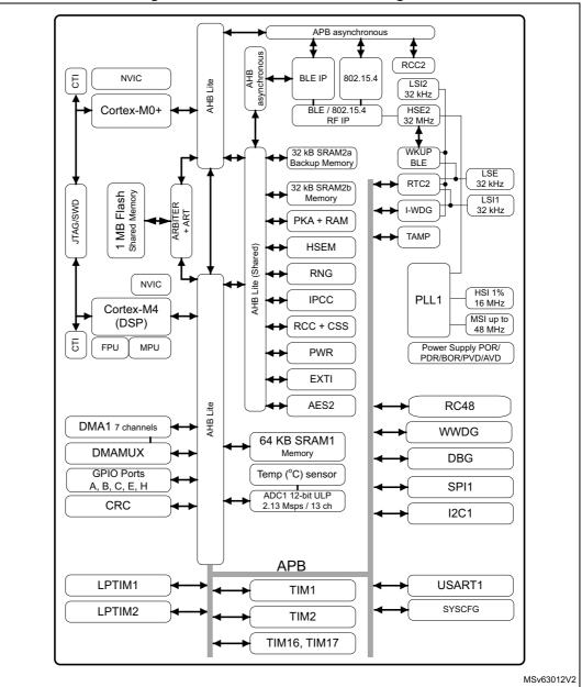
Figure 1. STM32WB50CGxx block diagram
