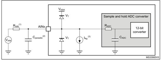
1. Refer to Table 70: ADC characteristics for the values of  $R_{AIN}$ ,  $R_{ADC}$  and  $C_{ADC}$ .
