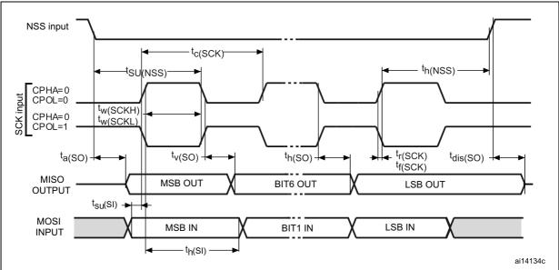
Figure 24. SPI timing diagram - slave mode and CPHA = 0
