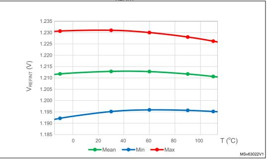
Figure 15. V<sub>REFINT</sub> vs. temperature
