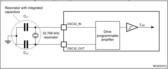
Figure 16. Typical application with a 32.768 kHz crystal
