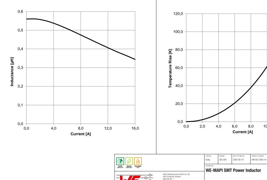
**Typical Temperature Rise vs. Current Characteristics:**
