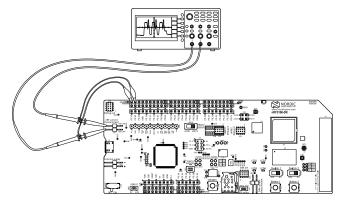
Figure 33: Current measurement with an oscilloscope
