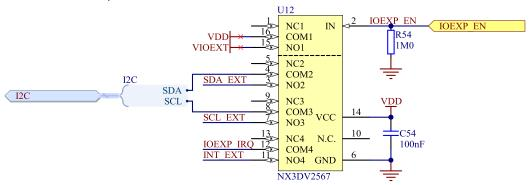
Figure 28: Switches for I/O expander
