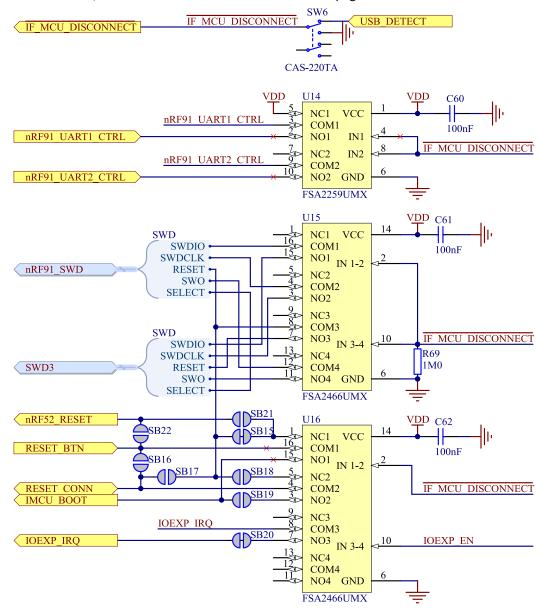
Figure 23: Signal interface switches
