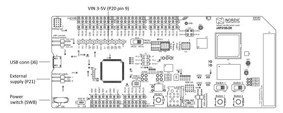
Figure 8: nRF9160 DK power supply options
