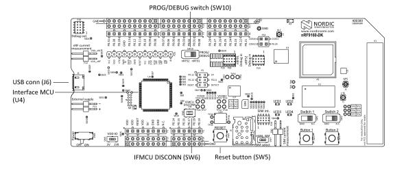
Figure 2: nRF9160 DK firmware development mode
