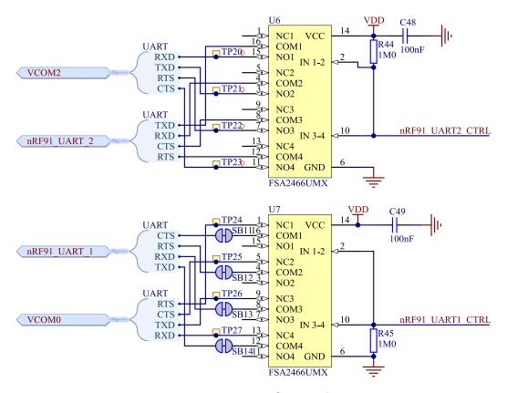
Figure 24: UART interface switches
