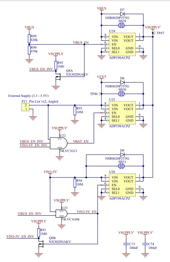
Figure 9: Power sources and switches
