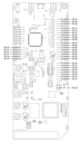
Figure 14: nRF9160 DK pins
