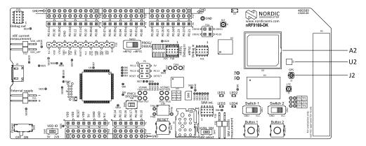
Figure 11: Onboard GPS antenna (A2), LNA (U2) and connector J2
