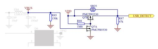
Figure 4: USB detect switch
