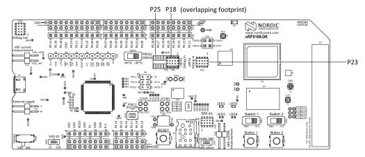
Figure 21: Debug input connector and trace footprint
