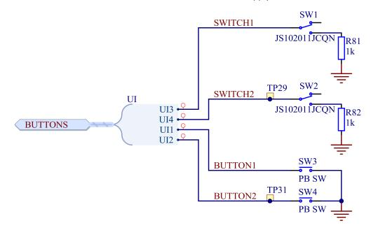
Figure 18: Buttons and switches
