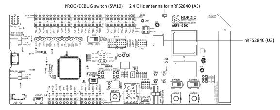
Figure 15: nRF52840 SoC on the nRF9160 DK
