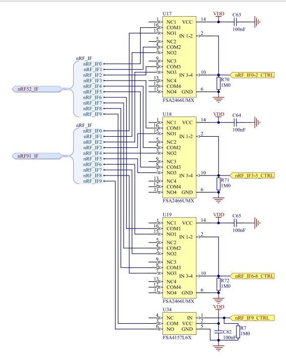
Figure 26: nRF52840 interface switches
