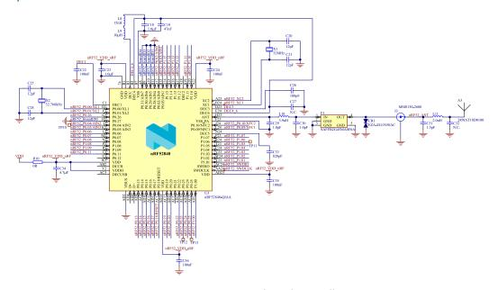
Figure 17: nRF52840 board controller
