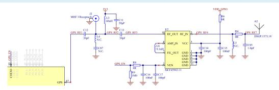
Figure 12: GPS connected to the nRF9160
