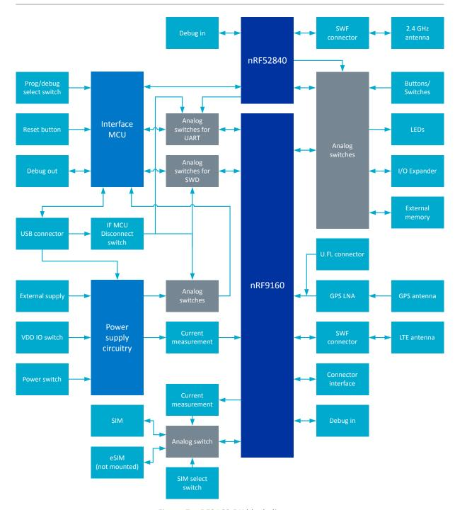
Figure 7: nRF9160 DK block diagram
