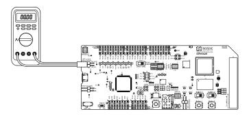
Figure 34: Current measurement with a current meter
