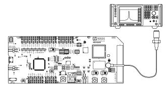
Figure 35: Connecting a spectrum analyzer
