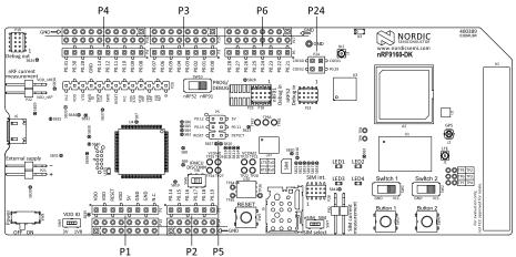
Figure 13: Access to nRF9160 GPIOs
