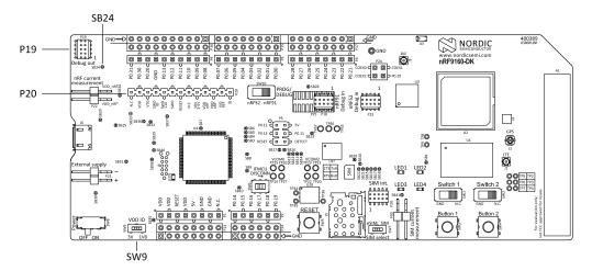
Figure 22: Debug output connector
