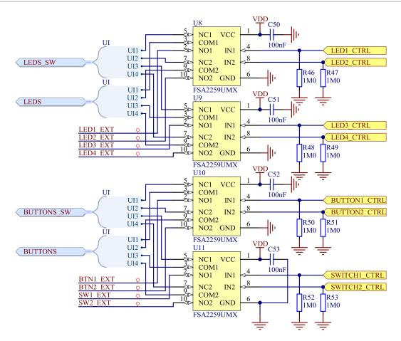
Figure 25: LED switch control
