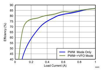
Figure 6. DC/DC Converter Light-Load Efficiency
