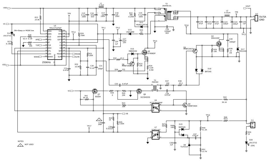
Figure 2. TPS23752EVM-145 Schematic (2)
