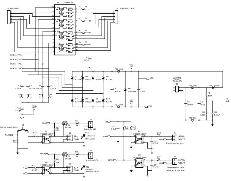
Figure 1. TPS23752EVM-145 Schematic
