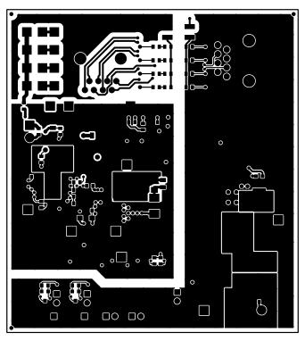
Figure 11. Bottom-Side Routing
