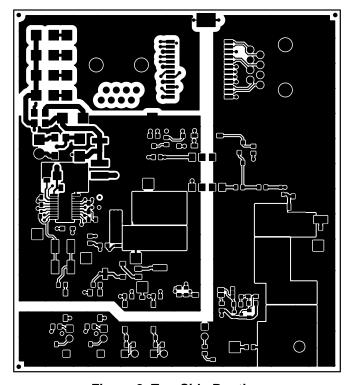
Figure 8. Top-Side Routing
