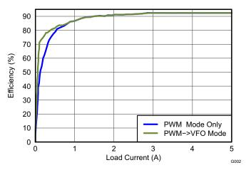
Figure 5. DC/DC Converter Efficiency
