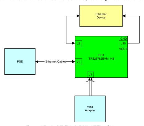
Figure 3. Typical TPS23752EVM-145 Test Setup
