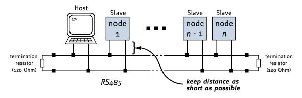
Figure 3: RS485 bus structure with termination resistors
