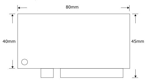
Figure 1: Board dimensions, position of mounting holes and position (pin 1) of connectors (all values in mm)
