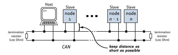
Figure 6: CAN bus structure with termination resistors
