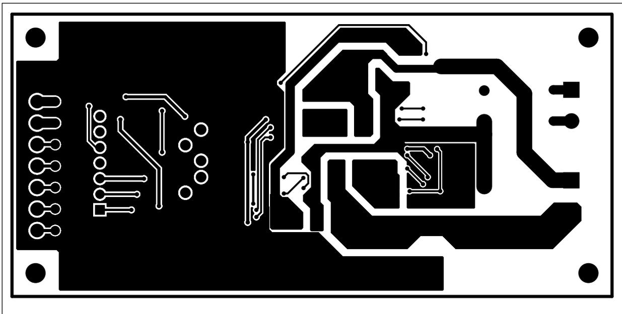
Figure 5. EVALPWD5F60 - layout (component placement view)
