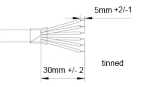
Figure 4-2 USBC-FS-UART-5V-5V-1800-WE Mechanical Details (dimensions in mm)
