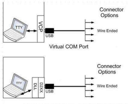
Software application access to USB via D2XX Figure 1-1 - Using the USBC-FS-UART-5V-5V-1800-WE
