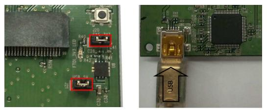
Figure 5. Supply 3V3 From Onboard LDO (J20, J21 Short)
