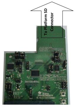
Figure 8. Connect to Platform With SDMMC for SDIO Interface
