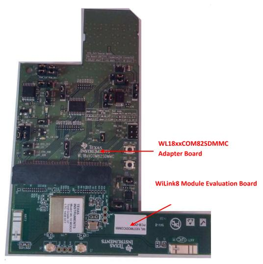
Figure 7. WiLink8 COM8 Board With Adapter Board Overview
