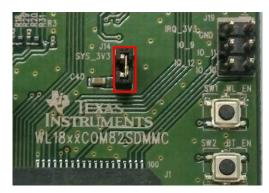
Figure 4. Supply 3V3 From FFC Connect (J14 Short)
