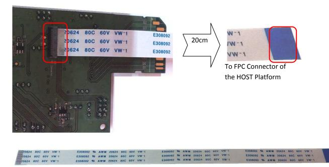
Figure 9. Connect to Platform With FPC Cable
