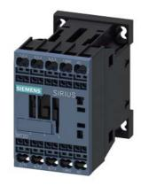
Power contactor, AC-3 9 A, 4 kW / 400 V 1 NO, 230 V AC, 50 / 60 Hz, 3-pole, Size S00 Spring-type terminal
