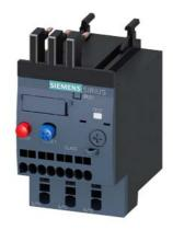
Overload relay 1.4...2.0 A Thermal For motor protection Size S00, Class 10 Contactor mounting Main circuit: Spring-type terminal Auxiliary circuit: spring-type terminal Manual-Automatic-Reset
