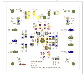
MAX20029B EV Kit Component Placement Guide—Top Assembly
