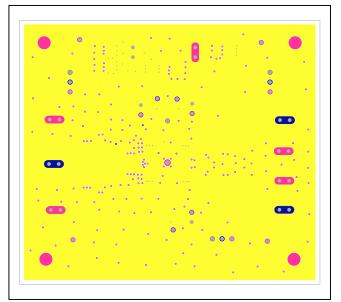
MAX20029B EV Kit PCB Layout—Inner Layer 2
