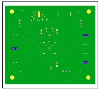
MAX20029B EV Kit PCB Layout—Inner Layer 1
