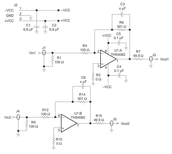
The gain of the EVM can easily be changed to support a particular application by simply changing the ratio of resistors R6 and R4 (channel 1) and R14 and R12 (channel 2) as described in the following equation:
