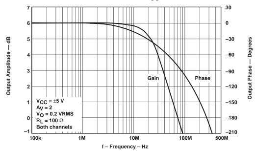
Figure 1–6. THS4062 EVM Frequency Response at  $V_{CC}$  =  $\pm$  5 V and Gain = 2
