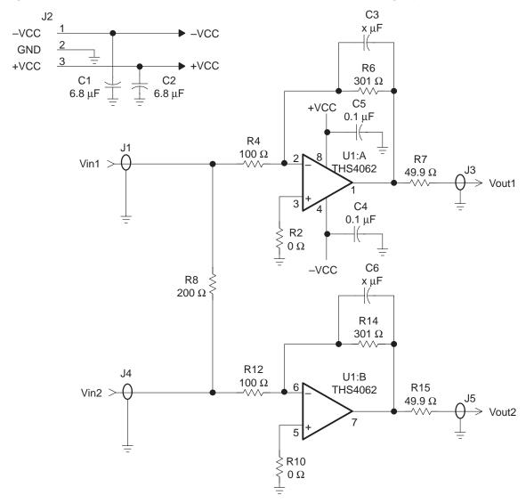
Figure 1–5. THS4062 EVM Schematic — Differential Input (Inverting Operation)
