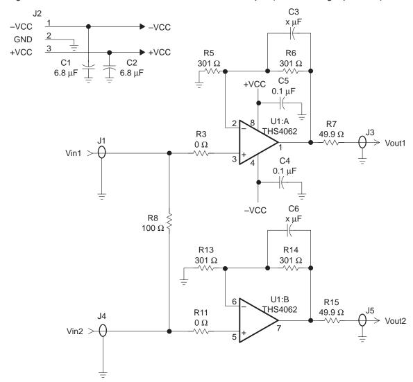
The gain of the EVM can easily be changed to support a particular application by simply changing the ratio of resistors R6 and R5 (channel 1) and R14 and R13 (channel 2) as described in the following equation:
