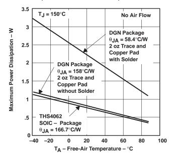
Even though the THS4062 EVM PCB is smaller than the one in the example above, the results should give an idea of how much power can be dissipated by the PowerPAD IC package. The THS4062 EVM is a good example of proper thermal management when using PowerPAD-mounted devices.
