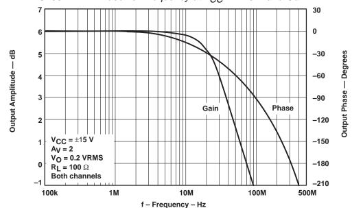
Figure 1–7. THS4062 EVM Phase vs. Frequency at  $V_{CC}$  =  $\pm$  15 V and Gain = 2
