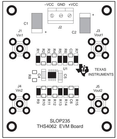
**Note:** The EVM is shipped with the following component locations empty: C3, C6, R2, R4, R8, R10, R12
