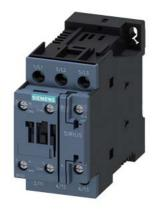
power contactor, AC-3 25 A, 11 kW / 400 V 1 NO + 1 NC, 24 V DC 3-pole, Size S0 screw terminal
