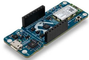
Power (XLP) PIC16LF18456 microcontroller, an ATECC608A CryptoAuthentication™ secure element and the RN4870 Bluetooth Low Energy Module.
