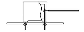
Temperature monitored inside the capacitor.
