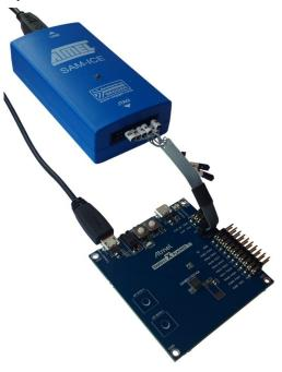
Figure 7-2. SAM-ICE using an Atmel-ICE Adapter
