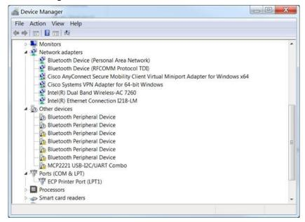
3. Right click MCP2221 USB-I2C/UART Combo device name and click Update Driver Software.... Figure 2-6. Update Driver Software
