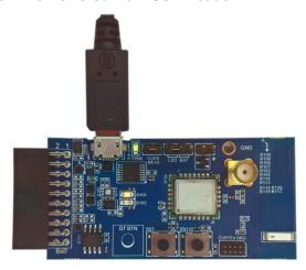
Any of the standard XPro Extension boards can be interfaced with the SAMR30 module XPro board using Xpander-XPro. The following is a sample image showing the reference for this setup.
