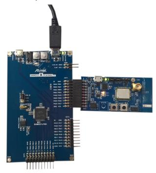
Initially, the XPro board must be programmed with the respective serial bridge firmware and the SAMR30 module XPro extension board must be programmed with Performance Analyzer firmware.
