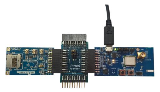
**Note:** Due to the limited number of available GPIOs in the ATSAMR30M18A module, few pins available in extension header of the board are multiplexed in the hardware through 0 Ohm resistors.
