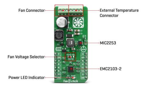
The EMC2103 includes an RPM based Fan Speed Control Algorithm. This fan control algorithm uses Proportional, Integral, and Derivative terms to automatically approach and maintain the system's desired fan speed to an accuracy directly proportional to the accuracy of the clock source.
