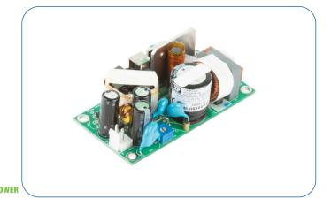
The ECF40 series is designed to minimize the no load power consumption and maximize efficiency to facilitate equipment design to meet the latest environmental legislation. Approved for medical and ITE applications in either Class I or Class II installations, this range of single output AC-DC power supplies are packaged in a low profile 1.1" height with a foot print of just 1.5" by 3". The ECF40 provides up to
