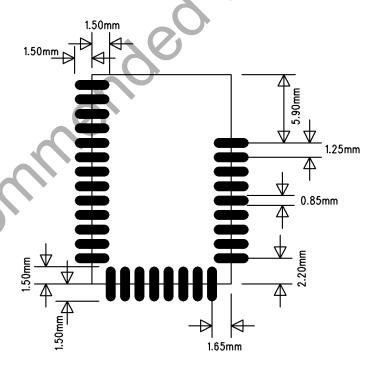
Figure 12: Recommended land pattern for BLE112-A and BLE112-E
