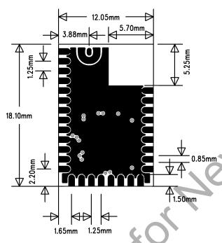
Figure 8: Physical dimensions and pinout (top view)
