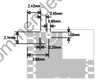
Figure 9: Dimensions for the RF pin
