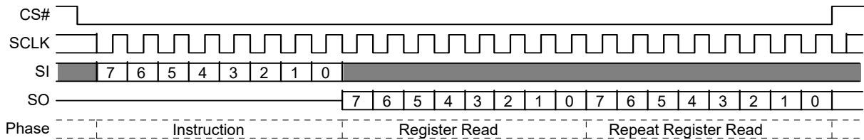
Figure 52. Read Configuration Register (RDCR) Command Sequence
