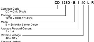
Forward Voltage \_\_\_\_ (Blank) = Standard L = Low
