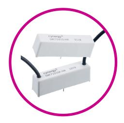
Very high isolation voltages, up to 15kV, are achieved through the use of high vacuum reed switches. Rhodium or tungsten contacts make these relays suitable for high reliability applications, such as cardiac defibrillators, test equipment and high voltage power supplies.
