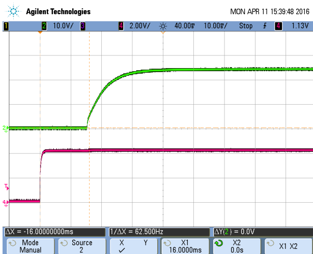
Turn-on transient at full load current (10 mS/div, Top Trace: Vout, 10V/div; Bottom Trace: ON/OFF, 2V/div)
