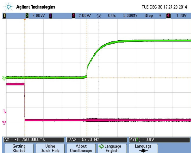
Turn-on transient at zero load current (5 mS/div, Top Trace: Vout, 2V/div; Bottom Trace: ON/OFF, 2V/div)
