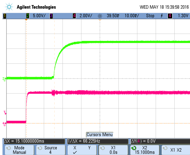
Turn-on transient at full load current (10 mS/div, Top Trace: Vout, 5V/div; Bottom Trace: ON/OFF, 2V/div)
