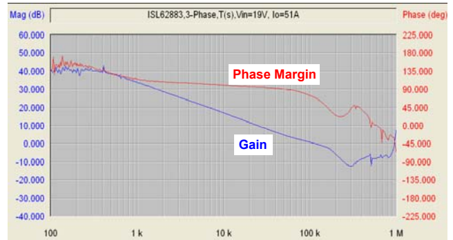
FIGURE 53. REFERENCE DESIGN LOOP GAIN T2(s) MEASUREMENT RESULT
