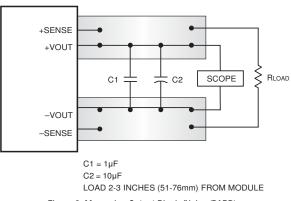
Figure 3. Measuring Output Ripple/Noise (PARD)
