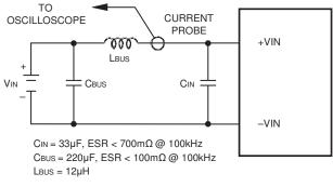
Figure 2. Measuring Input Ripple Current
