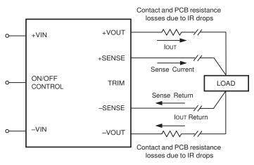
Figure 4. Remote Sense Circuit Configuration
