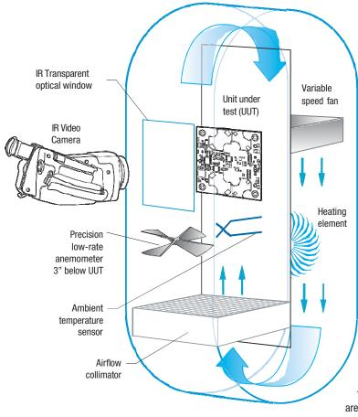
Figure 8. Vertical Wind Tunnel
