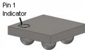
Figure 3. WLCSP Bumps Facing Down (Top View)
