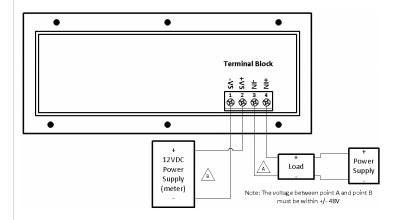
In this example, the load connects to terminals 3 and 4, where terminal 3 is the negative input terminal (-IN) and terminal 4 is the positive input terminal (+IN). The 12V power supply connects to terminals 1 and 2, where terminal 1 is the negative power supply terminal (-VS) and terminal 2 is the positive power supply terminal (+VS).
