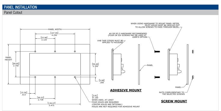
Note: When mounting panel meter with hardware, a four hole pattern (four outermost holes) or the six hole pattern may be used at the customer's option.
