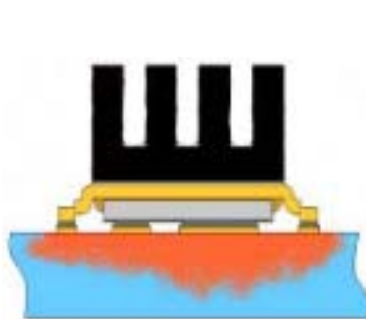
⑧ Mounted on minimum footprint full size board with metalized back and with small clip heatsink. (still air)
