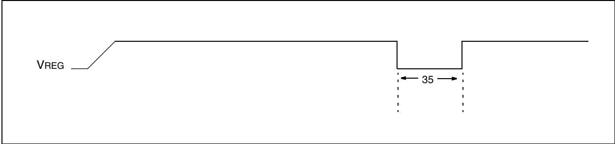
FIGURE 10-5: BROWN-OUT DETECT TIMING
