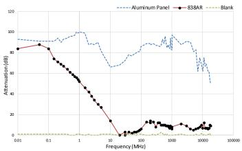
Test performed with a two-coat thickness.
